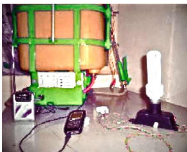
Fig-6: Applications of solar-powered sprayers for multiple uses
