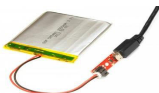
Fig7: Lithium Polymer Battery ARDUINO – INSTALLATION :
