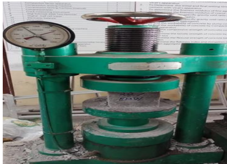
Fig. 6: Compressive strength testing of cube sample.
