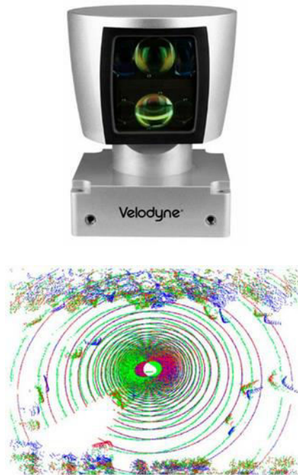
Figure 3.” A 3D-LiDAR sensor could be employed for short, medium, telescopic, or combinations (dual short range, dual medium) range. Here, a Velodyne HDL-64E sensor and its generated points cloud. (Images source: www.velodynelidar.com ; accessed on 29 October 2021).”
