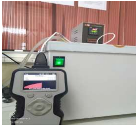
Figure 3. tempos Thermal Property Analyzer
