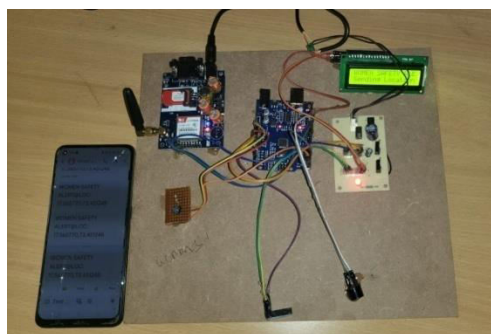
Fig 2: Hard ware kit of Women Safety Device with GPS Tracking Alerts.
