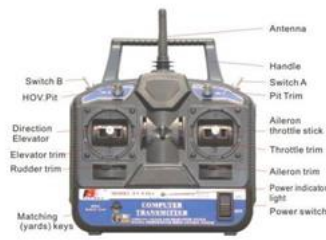
Figure: 10 Frequency transmitter
