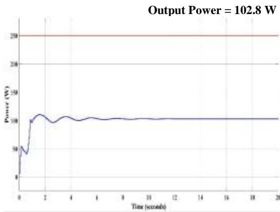
Fig.8: Tracking of maximum power with BOA
