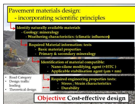
Figure 1: Recommended basic approach to road pavement materials design incorporating scientifically based concepts, developed for the selection of a material material compatible Newage (Nano) Modified Emulsion (NME) stabilising agent addressing the engineering requirements (physics) of a road pavement structure
