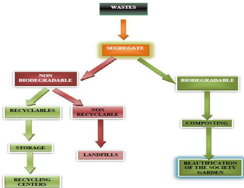
Figure 1: Diagrammatic Representation of the Solid Waste management Model of Housing Societies
