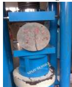
Fig 19. Split tensile strength test on cylinders
