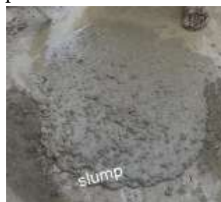
Fig 12 Slump Diameter measurement
