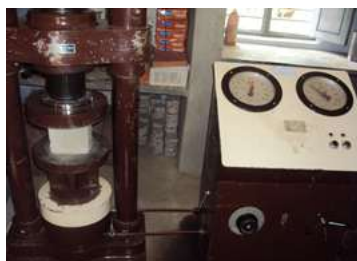
Fig 17. Compressive strength test on cubes
