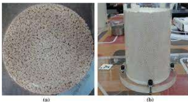
Fig 3. Perspectives of the double-porosity laterite soil: (a) Plane and (b) Front
