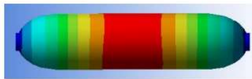
Figure 14. Schematic View of Mode Shape 2,
