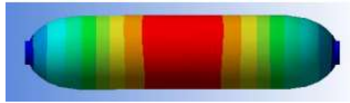
Figure 16. Schematic View of Mode Shape 3, Graphite [0/45/90/-45]s
