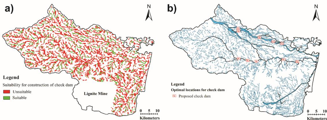
**Figure 9.** a) Suitable zone for construction of check dam b) Optimal sites proposed for construction of check dam
