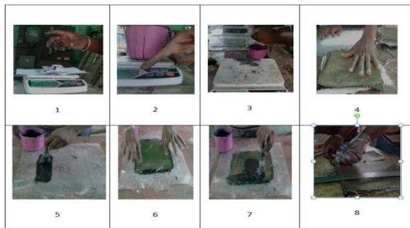
Figure 26 Complete sequential process for fabrication (1) Measuring mass of Epoxy resin (2) Measuring mass of Hardener (3) Taking appropriate proportion of Epoxy resin and Hardener (4) Measuring mass of fibers (5) Pouring of mixer into the mold (6) Applying pressure on mold (7) layering with epoxy resins and powders (8) Marking on specimen
