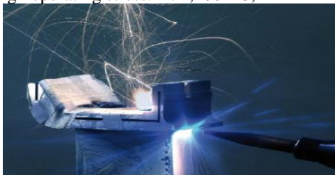
Figure 5: Turbine blade during laser drilling
