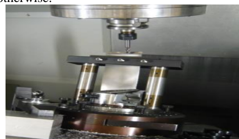
Figure 8: Adaptive CNC blending of repaired air foil tip
