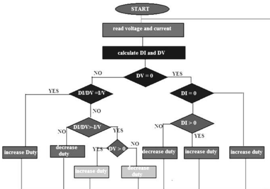
Flowchart of incremental conductance method
