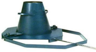
Fig 4.2: Slump Test in progress
