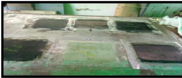
Figure 27 before cutting the specimen (curing period)
