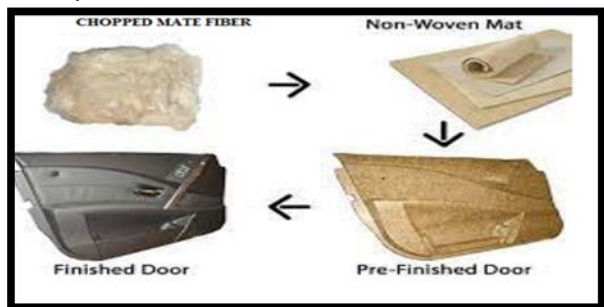
Figure 13 Bio composite cabin in car door, hoods, fans, and pipes, and extends even further. Polyester composites, endowed with innate
