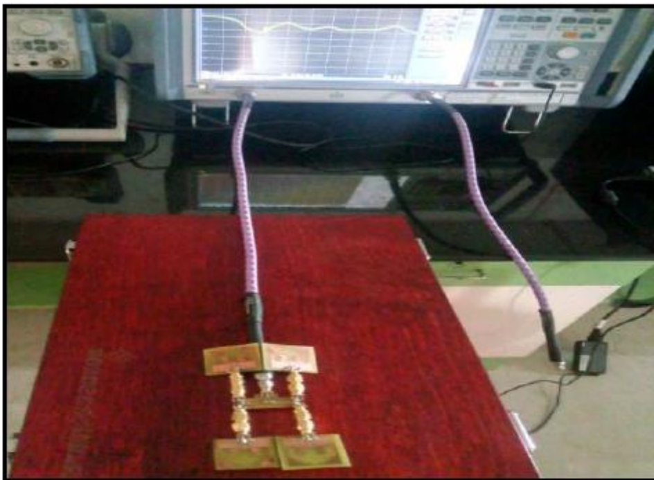
Fig. 18: Testing arrangement of proposed 1X4 Antenna Array using power divider
