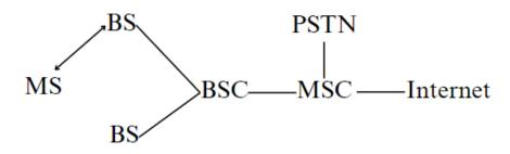
Figure 1. The architecture of AMPS
