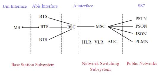
Figure 2. Architecture of the GSM System
