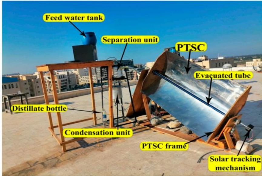
Fig 1. Photograph of test-rig.
