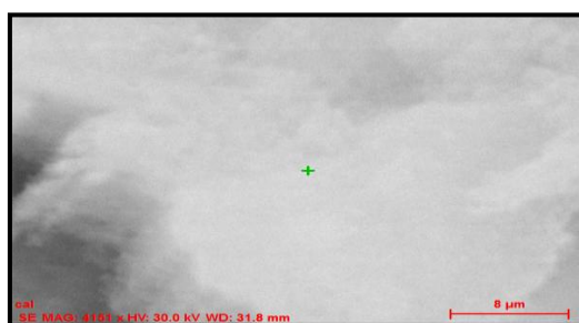
Figure 3: SEM analysis of carbon nanoparticles from Abrus seed oil, captured at 4150× magnification and 30.0 kV.
