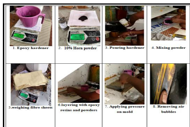
Figure 19 Complete sequential process for fabrication
