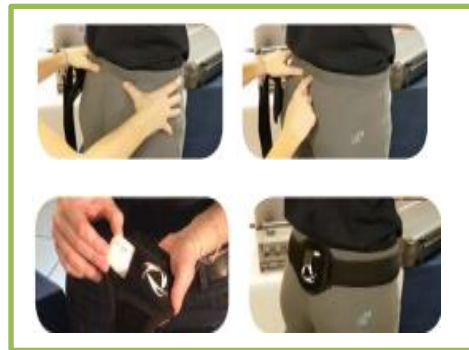
Figure 2. Insert the sensor inside the belt, with the flat part facing towards the back of the pocket.
