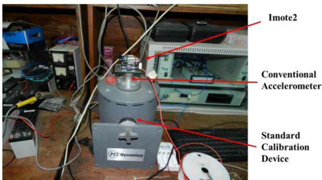
Figure 1. Imote2 The wireless sensor node is mounted on the accelerometer trim system
