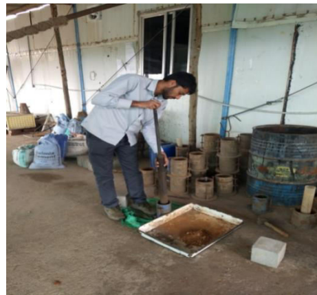
Fig 4.1.3: Conduction of Standard Proctor Test.
