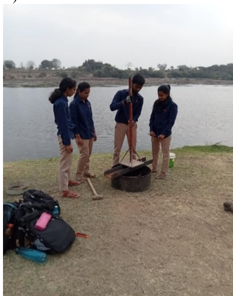
Fig 2.Setup infiltrometer on site
